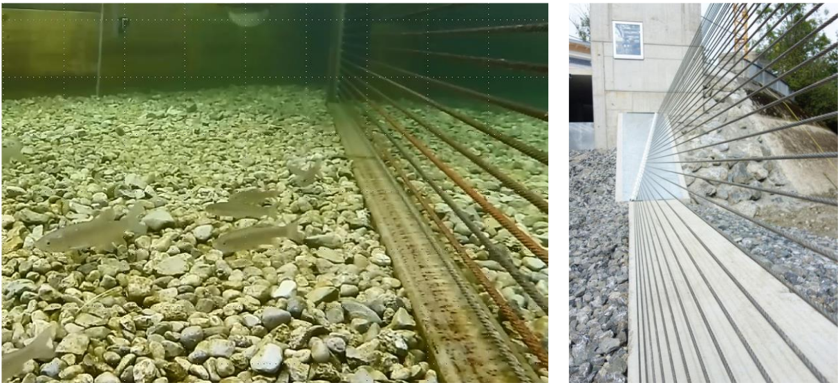
Fig. 8. Flexible FishProtector - installations in the ethohydraulic test (left) and in the first pilot project on a pre-Alpine river in Bavaria (right, during construction period in 2020).
